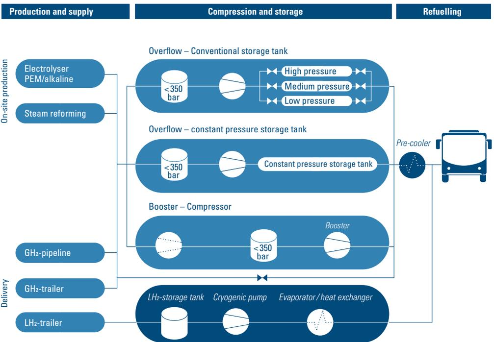
There are various supply concepts for the provision of hydrogen, which require a decision on a case-by-case basis. When hydrogen is delivered by lorry, it is either transported in gaseous form at 200–300 bar or in liquid form if there is a greater demand. If there is a hydrogen production plant in the immediate vicinity, it is possible to use a pipeline connection. Hydrogen can also be produced on site by means of an electrolyser.
