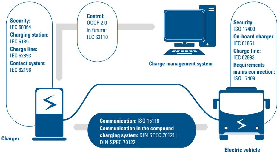
FIGURE 83 Overview of standardisation of conductive charging via docking system
